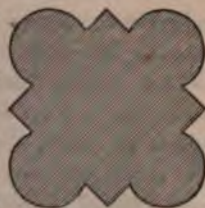
Section of Pier, St. Sennen Church.
